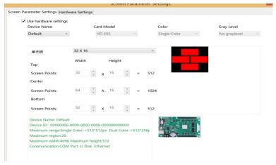
2). Cross sign screen can establish Global program and program, global program separated the top, middle and bottom and showing in one area. Establishing program can set up 3 areas to show program.
