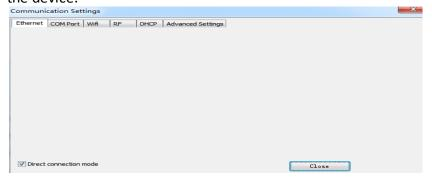
②.when not select "Direct connection mode", it is suitable for condition when controller and main operated PC are not at the same network segment, it need add the IP address of controller network segment to the software. Operation as below. After added, then you can find the controller in 192.168.3.\*
