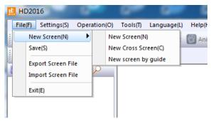
New screen (Ctrl+N): used to create a new screen, HD2016 manage screen without limited, can also be grouping manage(select group option in system setting). Save (Ctrl+S): used to save current screen file.
