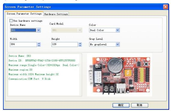
**2)** In Setting-screen parameter setting-hardware setting, if in commonly smart setting, it have the default screen parameter, then can direct choose, and click "sending".
