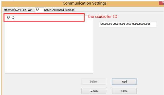
3). When all the device ID added to software, and connected all the control cards together, click Search, user can find all the control cards.
