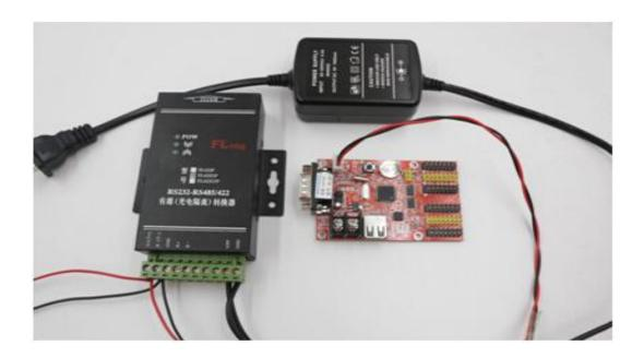
2). When first time connected multiple 485 communication card, one time only connect one card, then into HD2016 software communication setting interface click "search", Add control card ID to HD2016. As picture show: This operation it need one by one PCS control card
