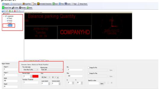
The initial state is from Max to Min, or from Min to Max. The decimal digit can set how much add or how much less. Also it can add the minimum and maximum values picture. The largest value can set to 9999999, decimal digits can set 3 numbers.
