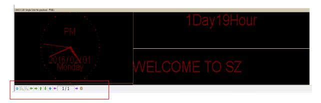
Notice: see the red place, there have tools for edit simulating screen. (Include tools: preview/pause preview, zoom in/ zoom out simulation window, current region right and left shift, region overall, display content paging, simulate display window top left corner display )
